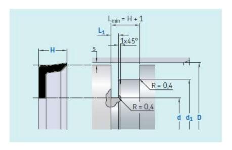
Since this is a non-standard seal profile no dimensions list is provided. We can custom design this seal to suit any existing housing.
